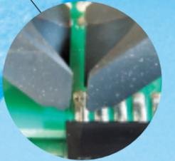
Soldering of flat cable or connectors
