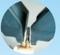
Soldering of coil wire
